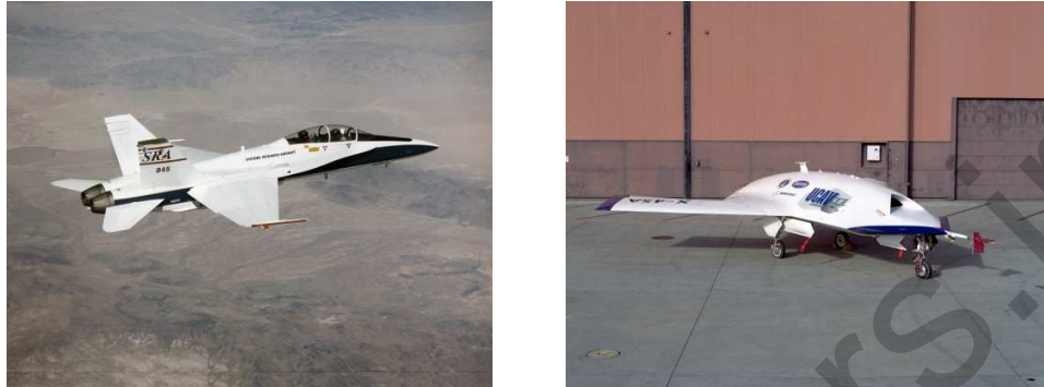
Figure 1.5: The F-18 aircraft, one of the first production military fighters to use “fly-by-wire” technology, and the X-45 (UCAV) unmanned aerial vehicle. Photographs courtesy of NASA Dryden Flight Research Center.
