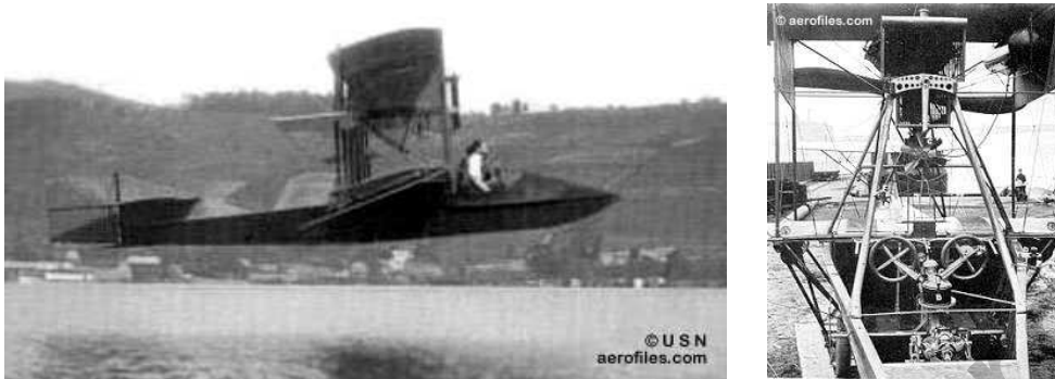
Figure 1.12: The Curtiss-Sperry E in 1912 (left) and a closeup of the Sperry Autopilot (right).
