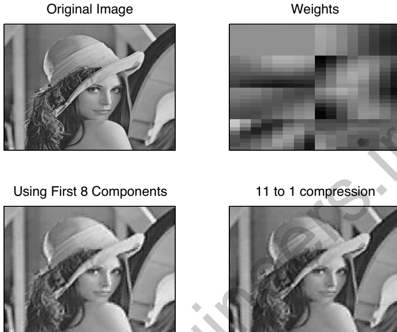
FIGURE 8.10 (a) An image of Lena used in the image-coding experiment. (b) 8 \times 8 masks representing the synaptic weights learned by the GHA. (c) Reconstructed image of Lena obtained using the dominant 8 principal components without quantization. (d) Reconstructed image of Lena with an 11-to-1 compression ratio using quantization.
