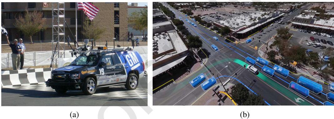
Figure 26.35 (a) Autonomous car BOSS which won the DARPA Urban Challenge. Photo by Tangi Quemener/AFP/Getty Images/Newscom. Courtesy of Sebastian Thrun. (b) Aerial view showing the perception and predictions of the Waymo autonomous car (white vehicle with green track). Other vehicles (blue boxes) and pedestrians (orange boxes) are shown with anticipated trajectories. Road/sidewalk boundaries are in yellow. Photo courtesy of Waymo.
