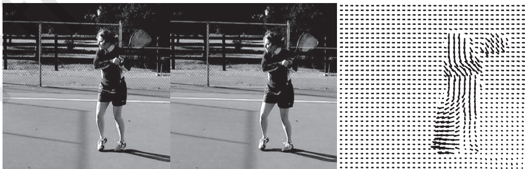
Figure 27.9 Two frames of a video sequence and the optical flow field corresponding to the displacement from one frame to the other. Note how the movement of the tennis racket and the front leg is captured by the directions of the arrows. (Images courtesy of Thomas Brox.)
