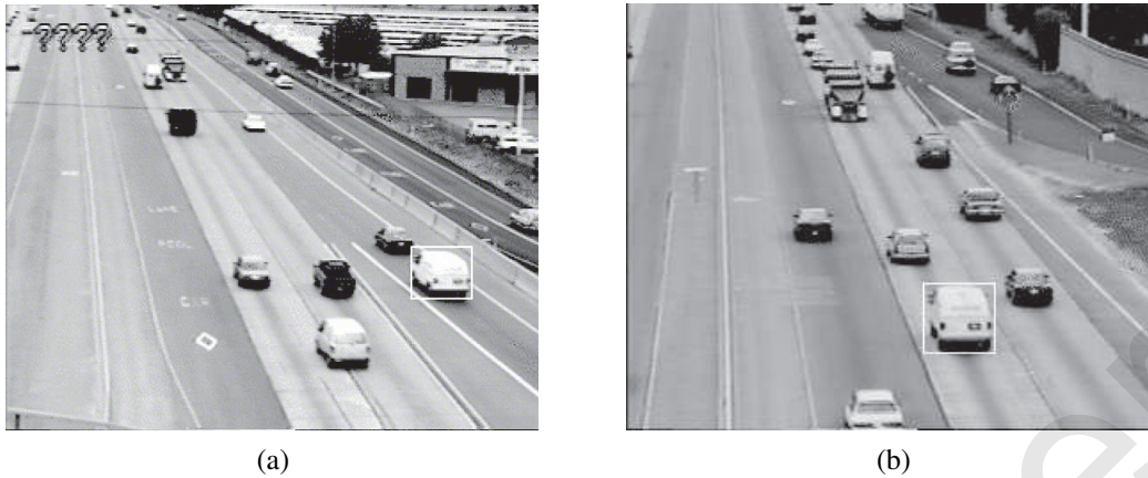
Figure 18.10 Images from (a) upstream and (b) downstream surveillance cameras roughly two miles apart on Highway 99 in Sacramento, California. The boxed vehicle has been identified at both cameras.
