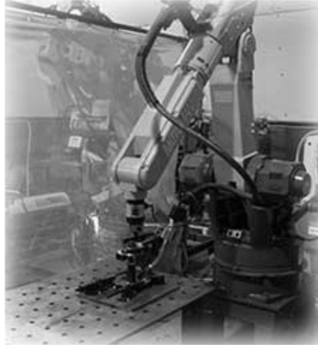
FIGURE 17.9 Robot Performing Drilling Operation.
