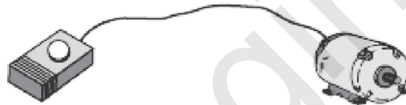
(In a traditional system, all control devices are wired directly to each other)
