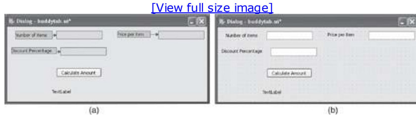
Figure 7.20. (a) Widgets on the form with the buddies set. (b) The dialog in Widget Editing mode.
