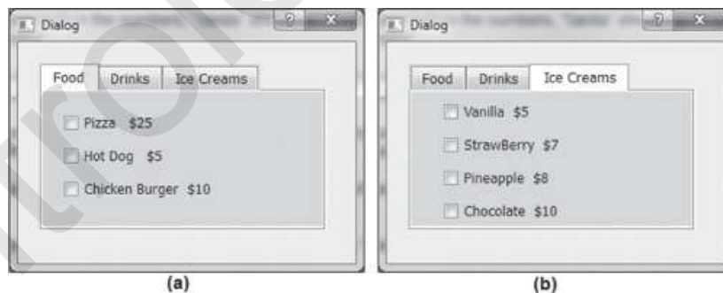
Figure 10.28. (a) The tab contents of the Food Tab button. (b) The tab contents of the Ice Creams Tab button.
