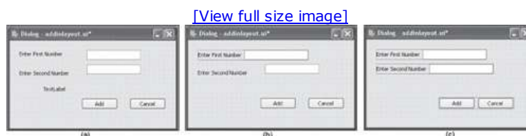
Figure 11.6. (a) Initial layout of the widgets. (b) Label and the first Line Edit arranged in horizontal layout. (c) All widget pairs arranged in horizontal layout.
