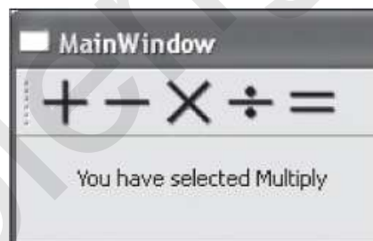
Figure 10.13. The toolbar displaying different toolbar buttons and a Label widget indicating the button that is selected.
