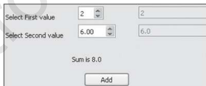
Figure 8.7. The spin box and double spin box values displayed through LineEdit along with their sum.
