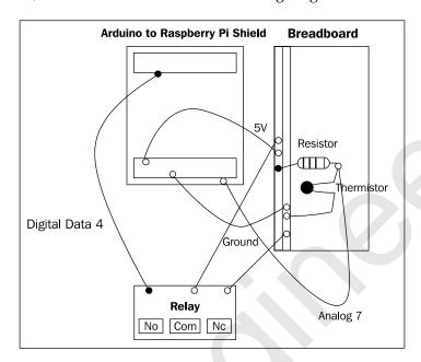
This circuit makes up the core of our thermostat. For the moment, we will not connect the fan to the relay but work on the software needed to run the thermostat.
